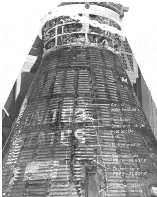
Fig. 23 Effects of reentry heating on the Gemini II spacecraft. From [40] (or [39]).
